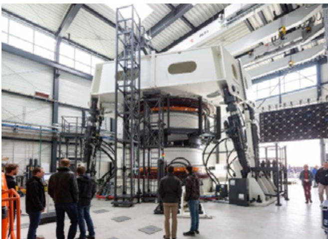
Test benches like this one for large bearings at Fraunhofer IWES in Hamburg are available for testing wind propulsion systems on ships
